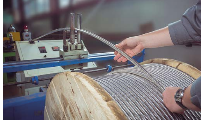
Stahlmann corrugated tube fed for annealing
