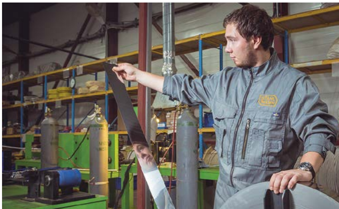
304 and 316L stainless steel strip used in the manufacture of corrugated tubes
